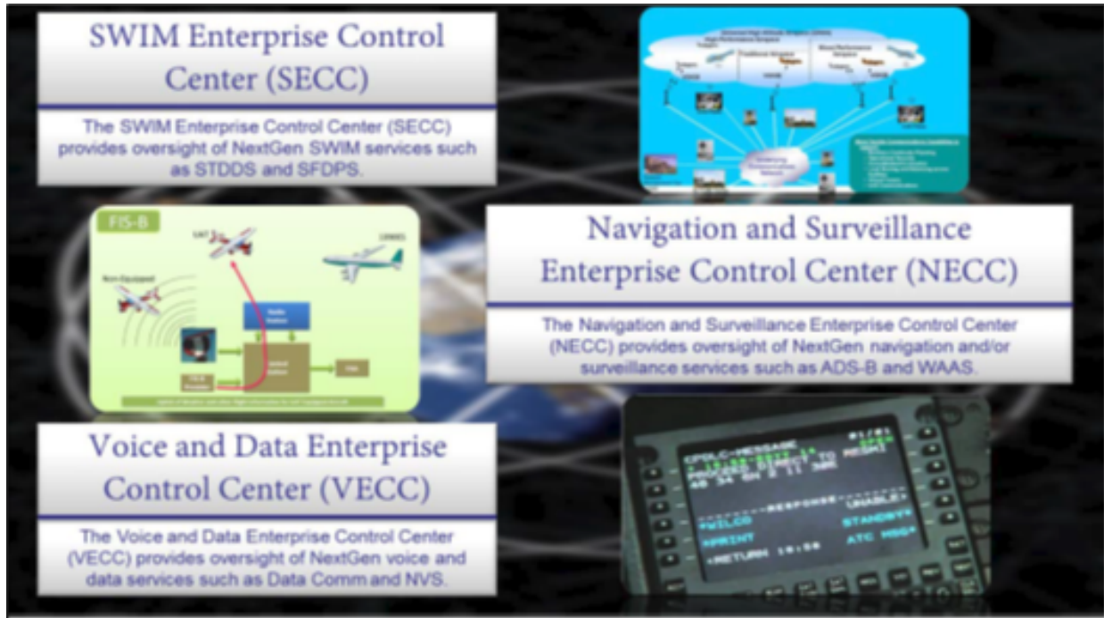
Fig. 2. Enterprise Control Centers and Data Services - The three-core center which makes up the FAA digital enterprise and services provided to aviation consumers. The screenshot image is captured from the FAA's ATO CyberDayBriefing in 2020.
