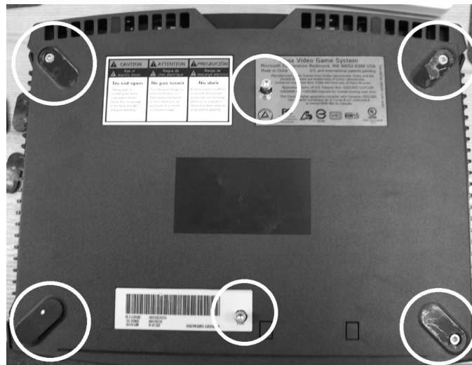
Figure 1. Xbox screw locations.
