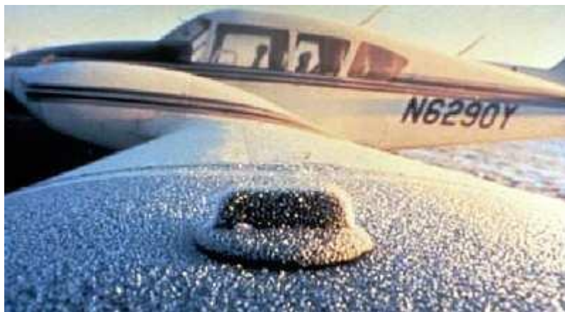
Figure 5: upper surface ice in flight.
