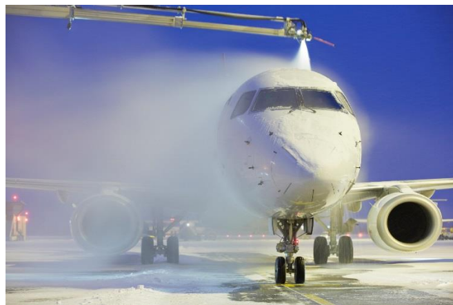
Figure 7: ice prevention before flight.
