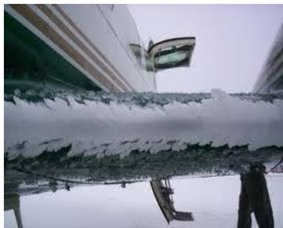
Figure 4: leading edge ice build-up on a wing.
