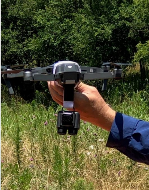
DJI Mavic Pro with Ion Cub PID attached directly below the sUAS
