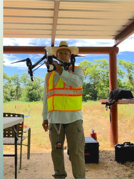
DJI Inspire 1 with Ion Cub PID attached with a short tether
