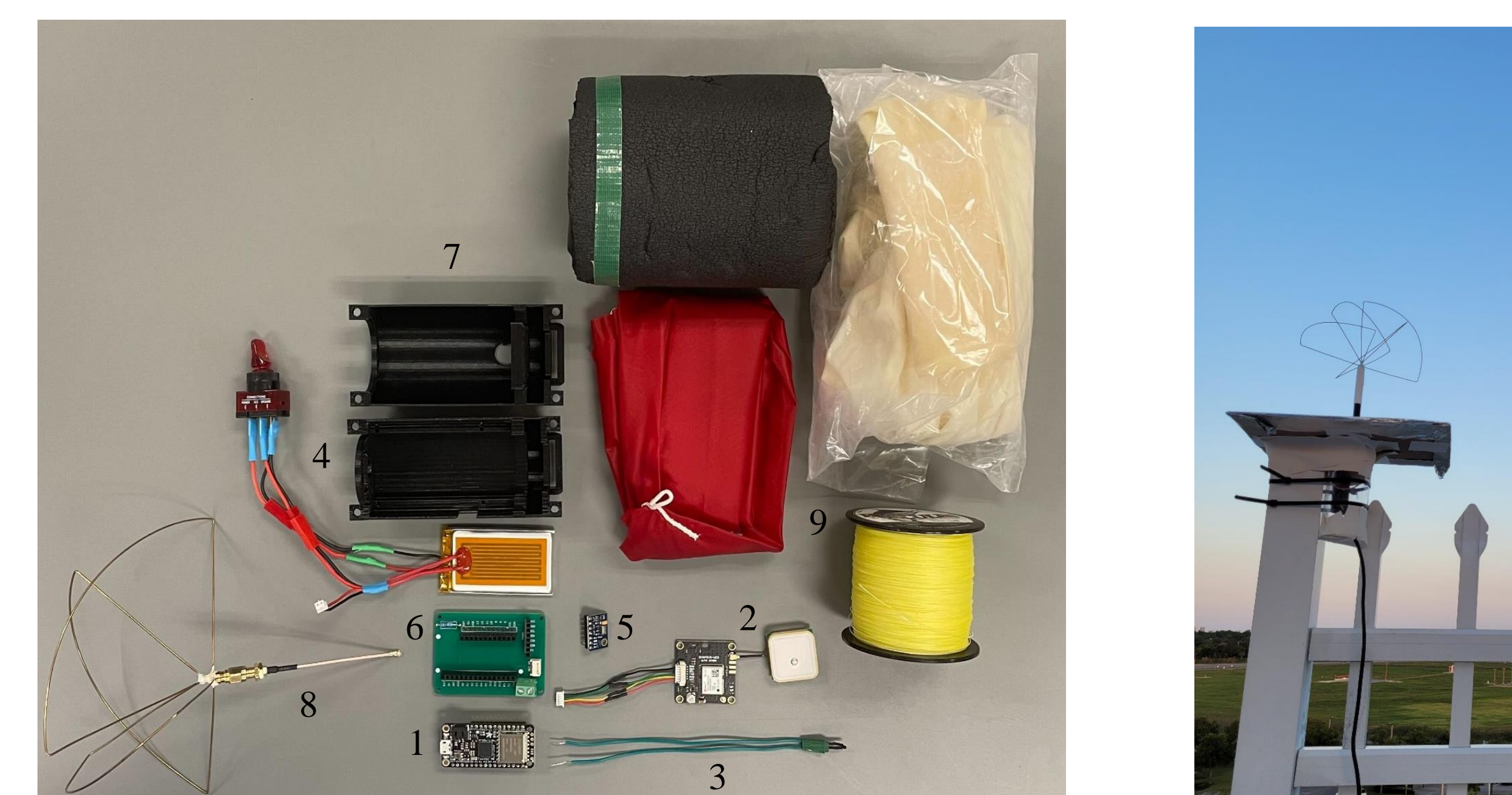
Material layout of all components needed to build and fly a GPSsonde (left) and fully assembled ground station built and ready to receive data (right)
